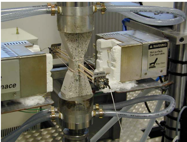
Fig. 5. Tensile test device: zoom on the active parts.
